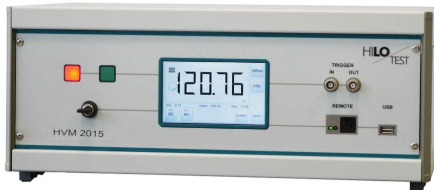
The high-voltage measurement instruments HVM 2015 consist of a measuring amplifier for universal use with a digital touch display, a built-in high-voltage divider for direct measurement up to 10 kV / optional 20 kV and an external input for an external high-voltage divider, HVT\*\*\*RCR, measurement and display of voltages up to 300 kV.
